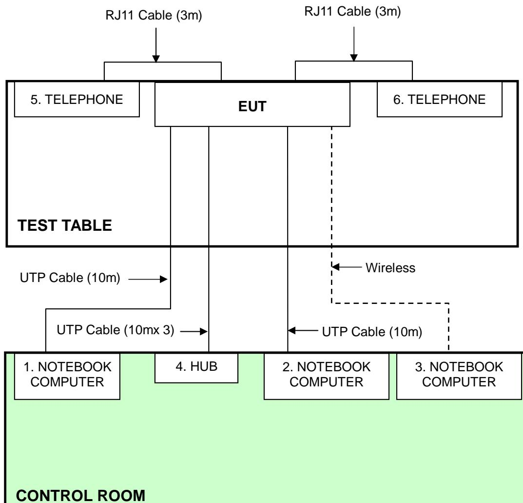
**NOTE:** 1. Support units 1-4 were kept in the control room during the test.
