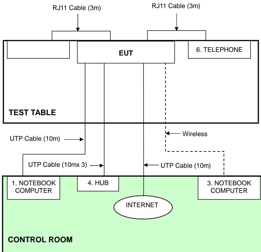
**NOTE:** 1. Support units 1, 3 and 4 were kept in the control room during the test.
