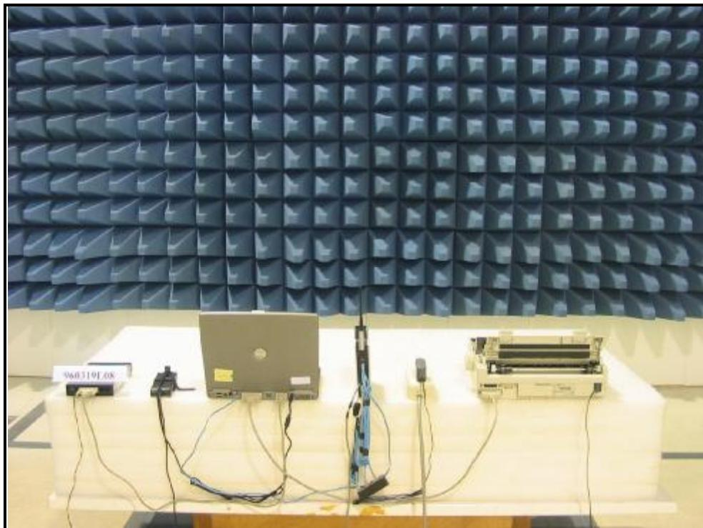
RADIATED EMISSION BELOW 1GHz TEST (Test Mode D)
