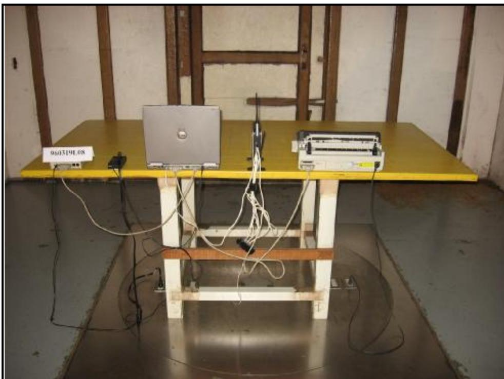
RADIATED EMISSION ABOVE 1GHz TEST (Test Mode D)
