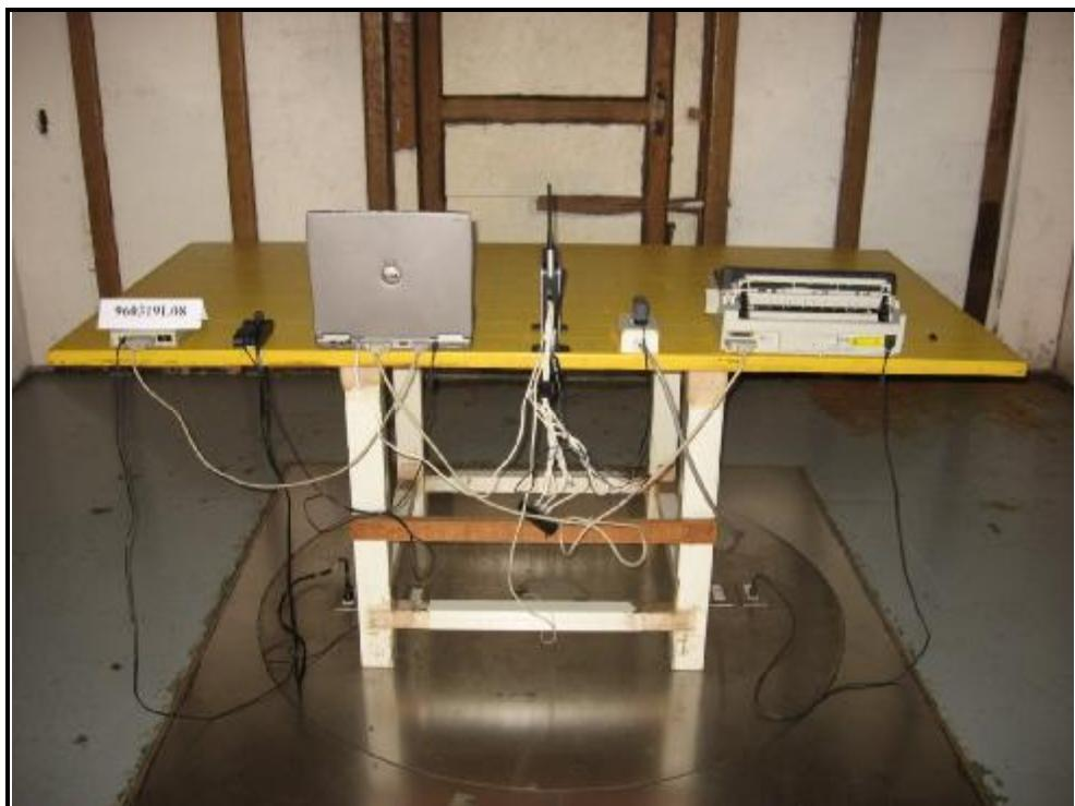
RADIATED EMISSION ABOVE 1GHz TEST (Test Mode C)
