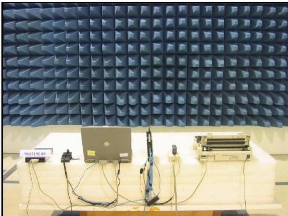
RADIATED EMISSION BELOW 1GHz TEST (Test Mode C)
