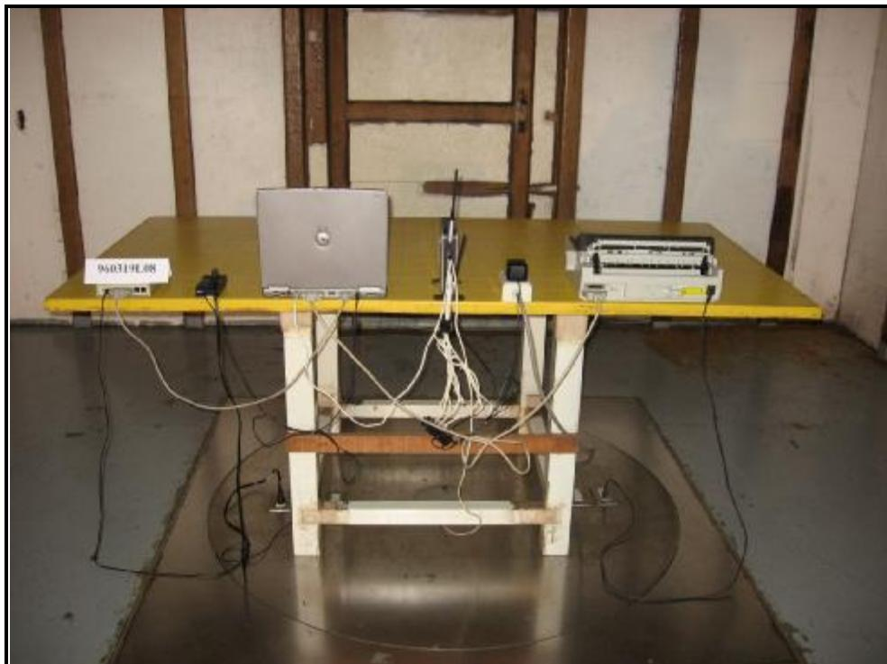
RADIATED EMISSION ABOVE 1GHz TEST (Test Mode A)
