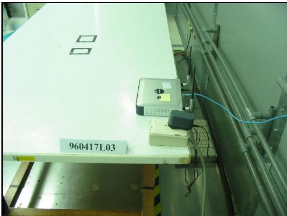
CONDUCTED EMISSION TEST (Test Mode B)
