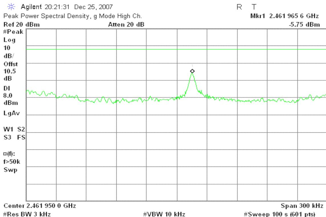
**draft 802.11n Standard-20 MHz Channel mode / Chain 0****PPSD (CH Low)**
