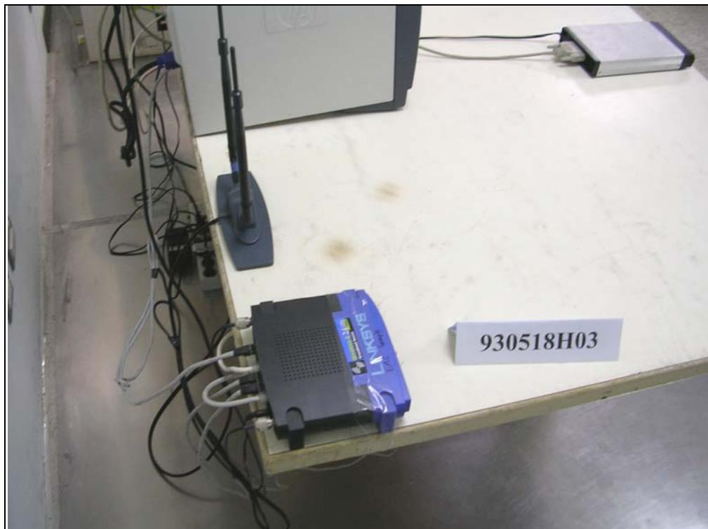
**CONDUCTED EMISSION TEST (antenna without the remote antenna-stand)**
