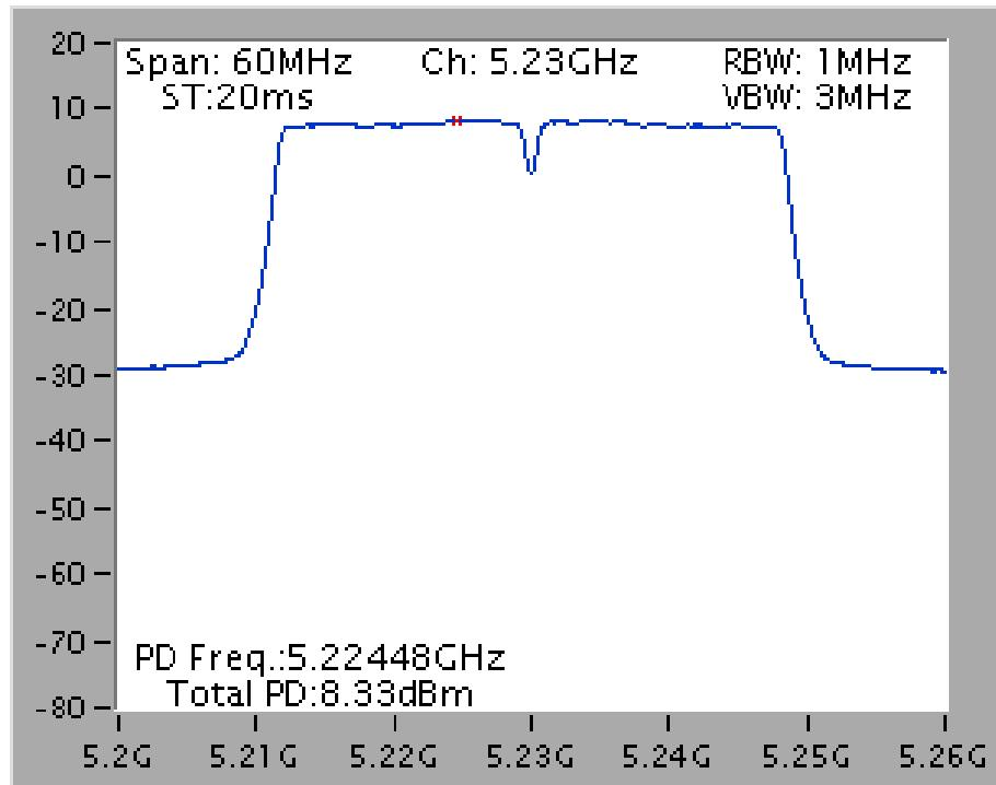
Power Density Plot on Configuration IEEE 802.11ac MCS0/Nss1 VHT80 / Ant. 1 + Ant. 2 + Ant. 3 / 5210 MHz
