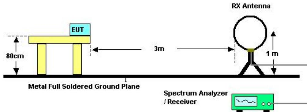
For Radiated Emissions: 30MHz~1GHz
