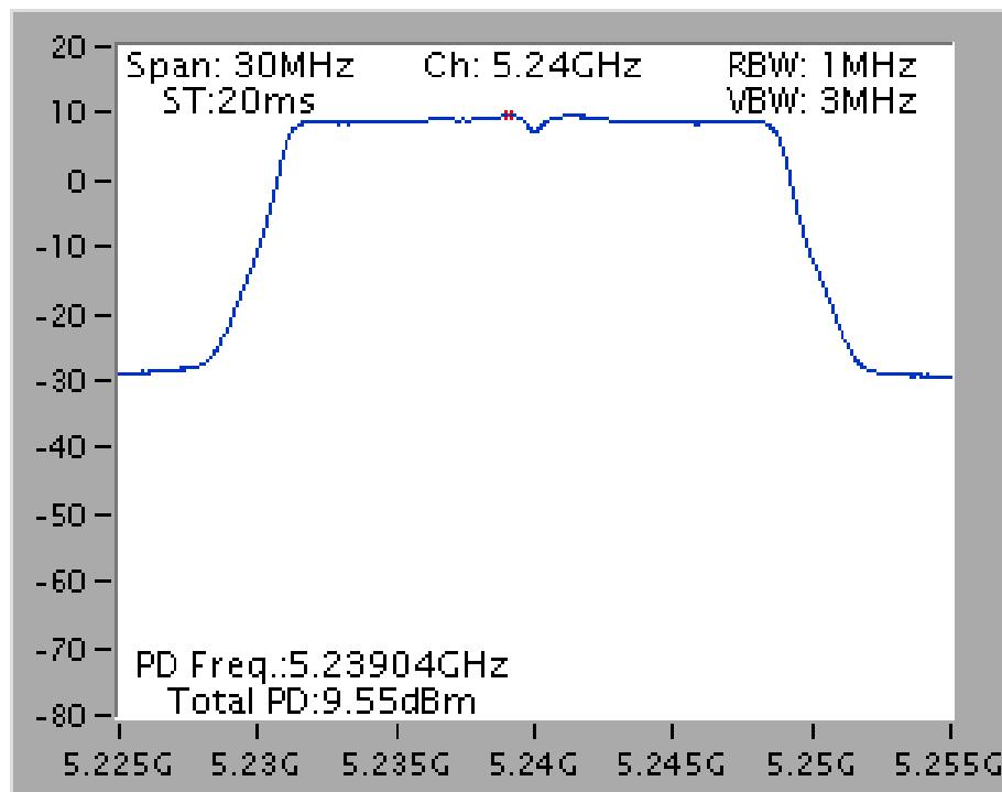
**Power Density Plot on Configuration IEEE 802.11ac MCS0/Nss1 VHT40 / Ant. 1 + Ant. 2 + Ant. 3 / 5230 MHz**
