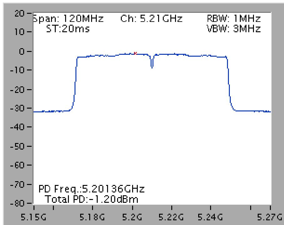
Power Density Plot on Configuration IEEE 802.11a / Ant. 1 / 5240 MHz
