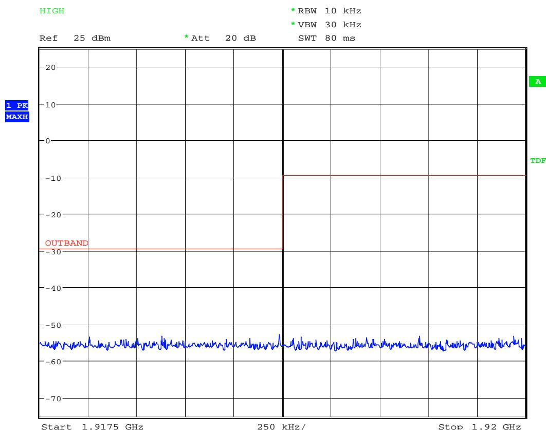
**Out-of-band Unwanted Emissions: CH FH****Higher band-edge**
