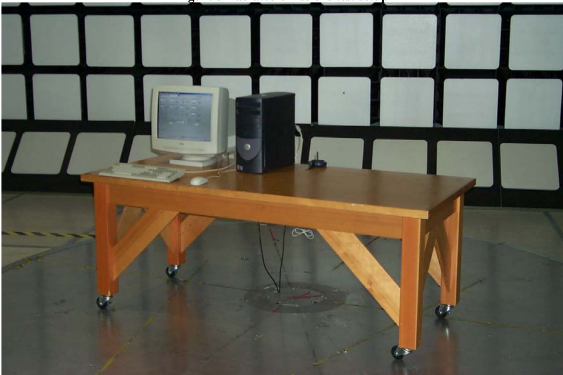
Figure 4 Radiated emissions test setup
