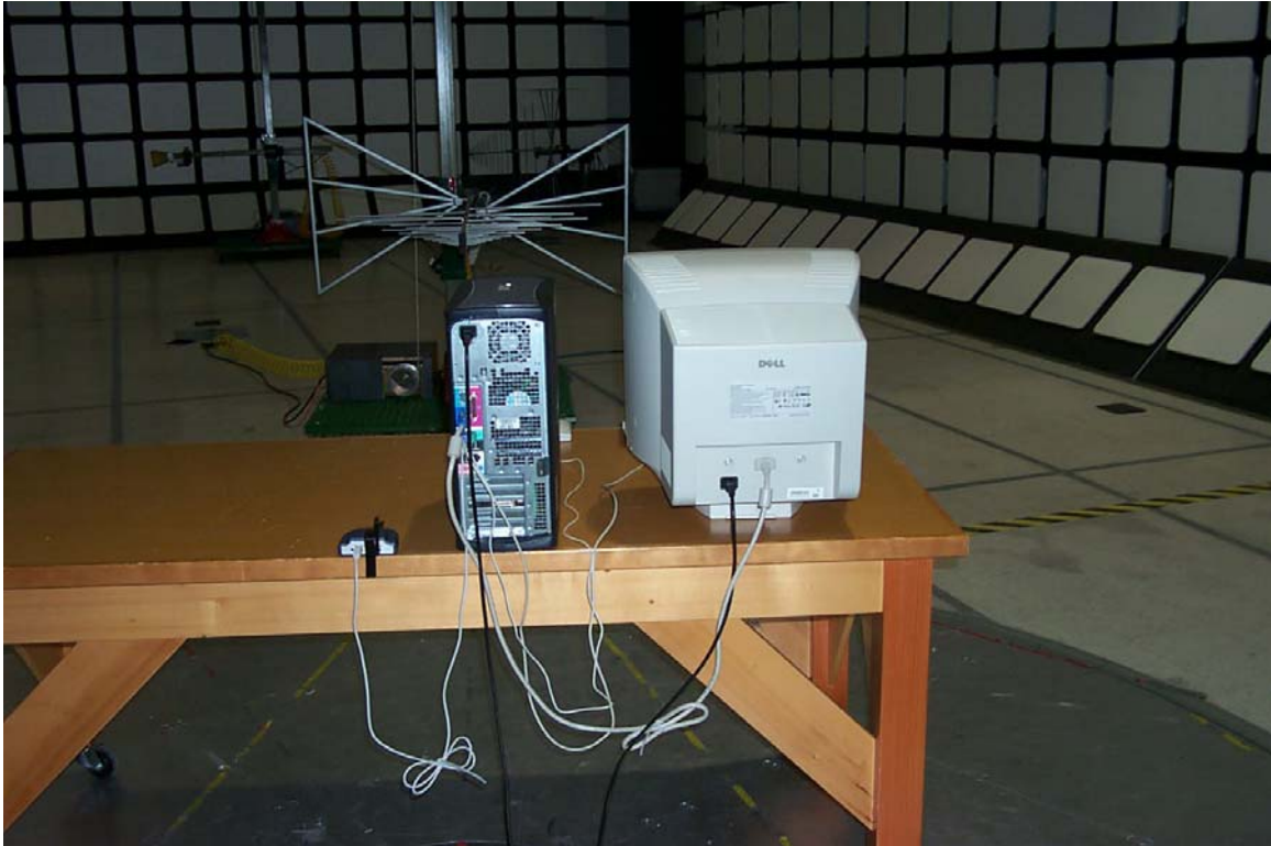
Figure 3 Radiated emissions test setup
