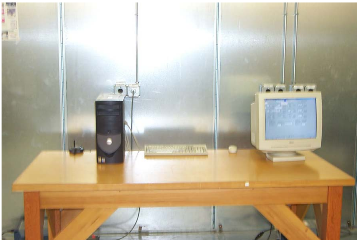
Figure 1 Conducted emissions test configuration
