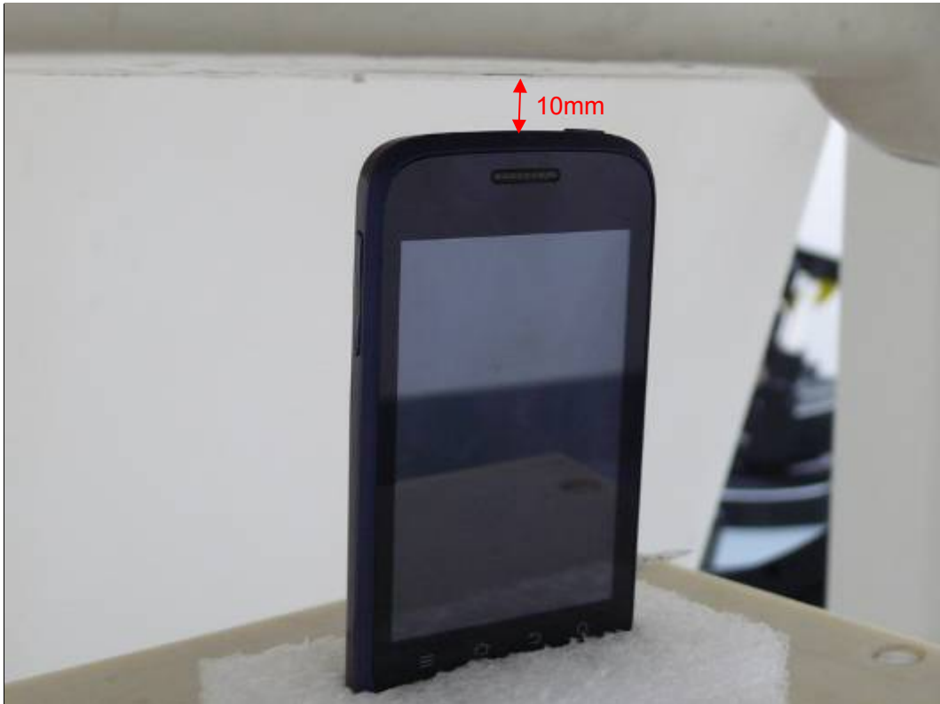
Picture 19: Top Edge, the distance from handset to the bottom of the Phantom is 10mm
