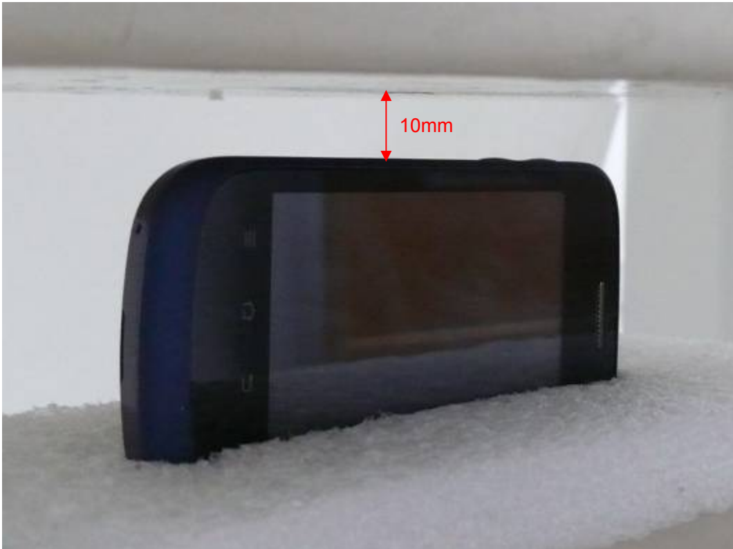
Picture 17: Left Edge, the distance from handset to the bottom of the Phantom is 10mm
