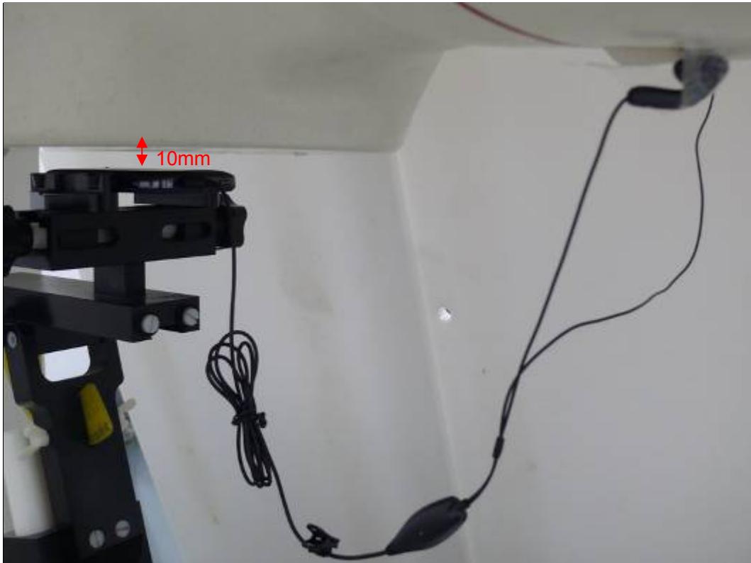
Picture 21: Back Side with earphone, the distance from handset to the bottom of the Phantom is 10mm
