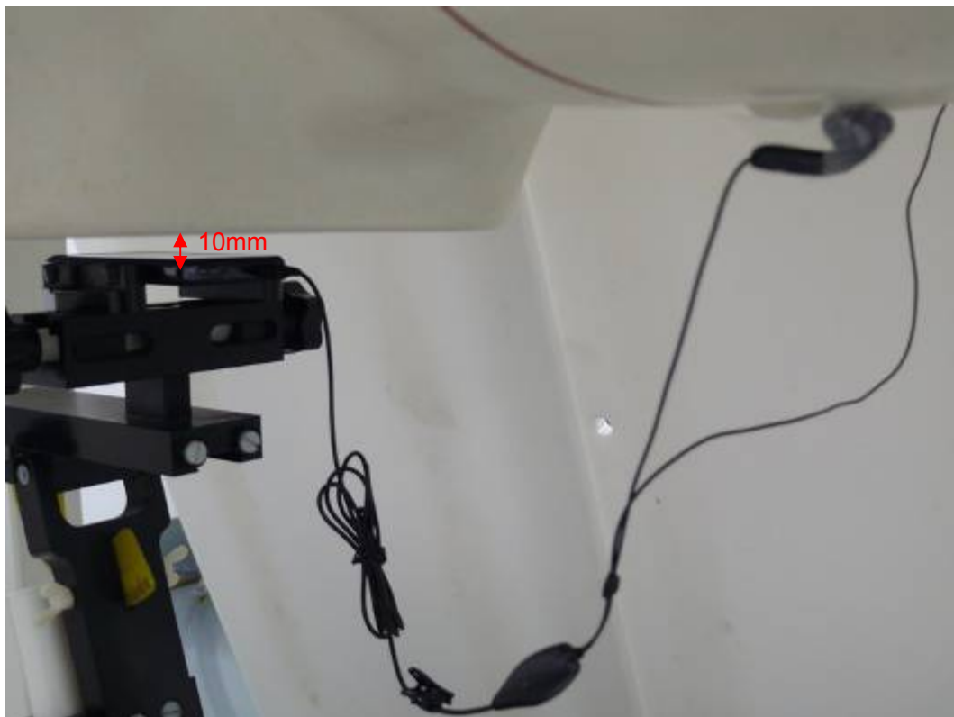
Picture 22: Front Side with earphone, the distance from handset to the bottom of the Phantom is 10mm
