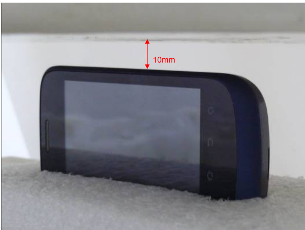
Picture 18: Right Edge, the distance from handset to the bottom of the Phantom is 10mm
