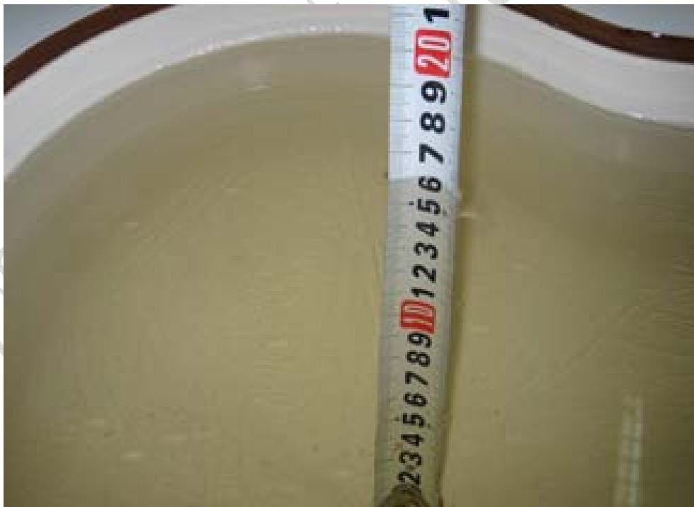
Picture 8 Liquid Depth at Ear Reference Point for 835MHz Head Liquid
