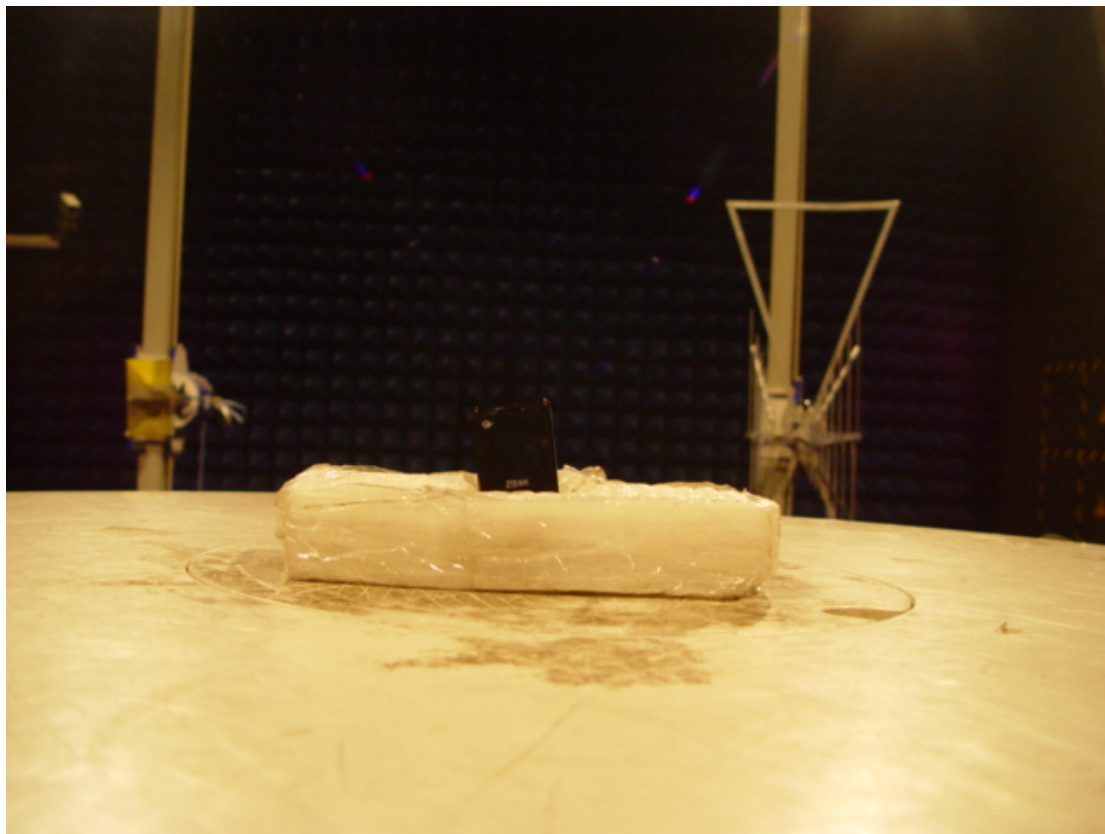
Radiated Spurious Emissions Test setup
