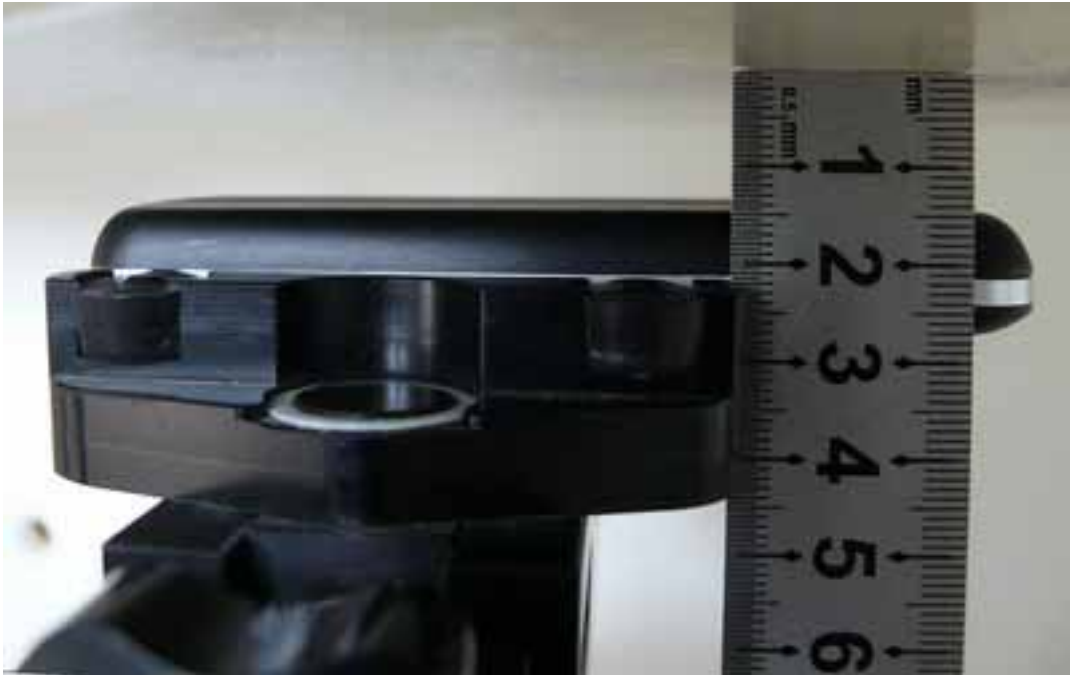
Picture 11: Body, The EUT display towards ground, the distance from handset to the bottom of the Phantom is 15mm)
