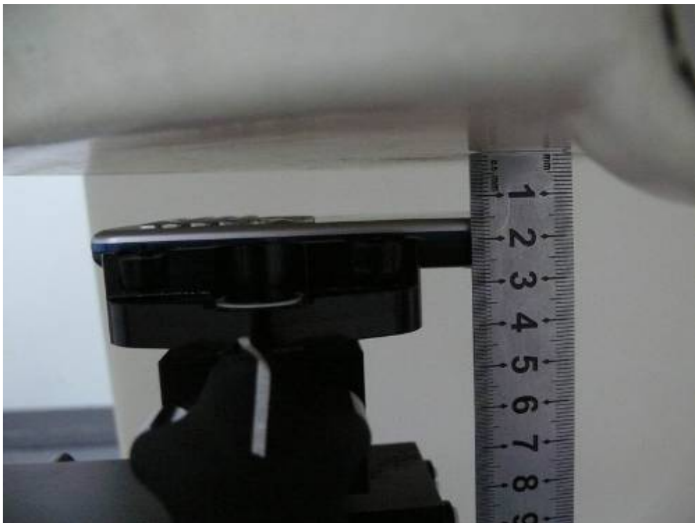
Picture 13: Body, The EUT display towards phantom, the distance from handset to the bottom of the Phantom is 15mm
