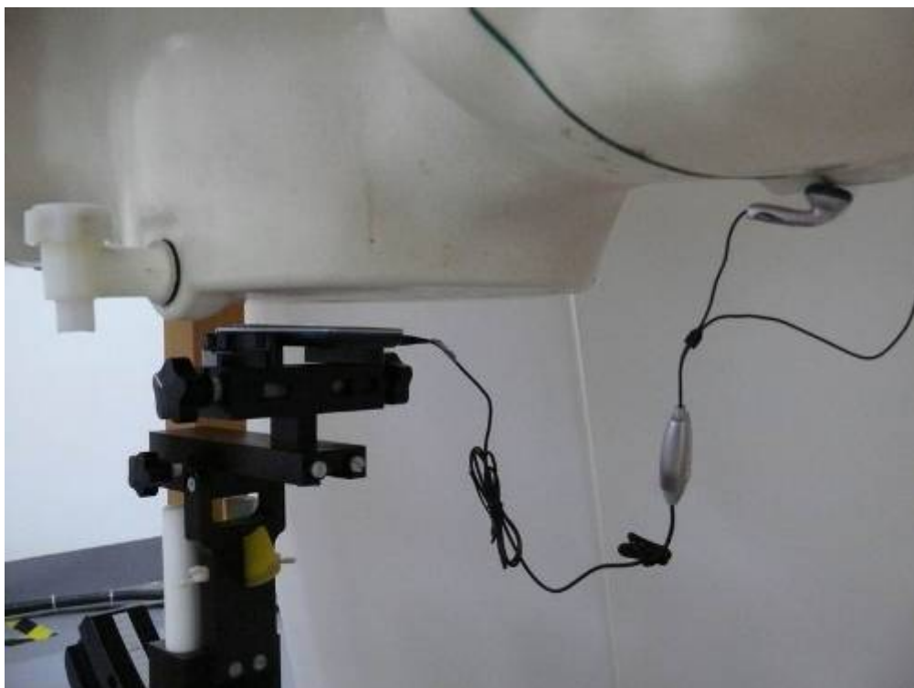
Picture 15: Body with earphone, The EUT display towards phantom, the distance from handset to the bottom of the Phantom is 15mm
