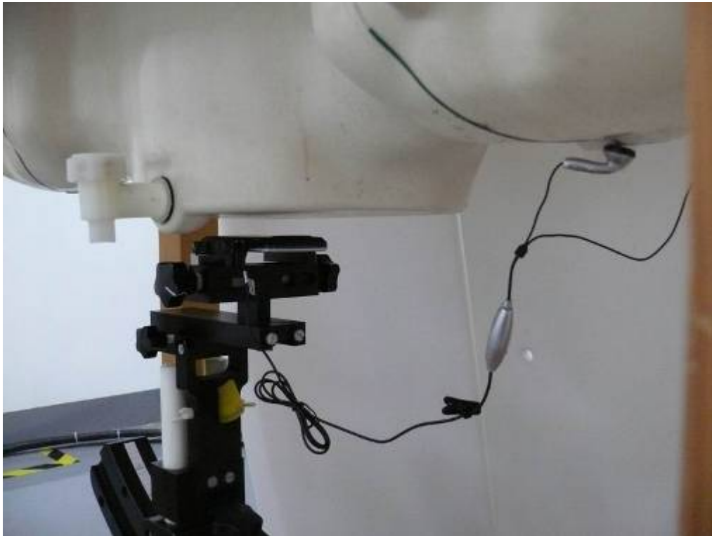
Picture 14: Body with earphone, The EUT display towards ground, the distance from handset to the bottom of the Phantom is 15mm
