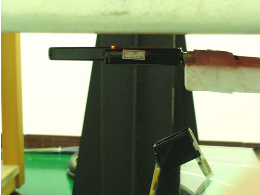
USB Configuration 2 with 10 mm separation for Back-Off SAR (Ant. set 180 degree)
