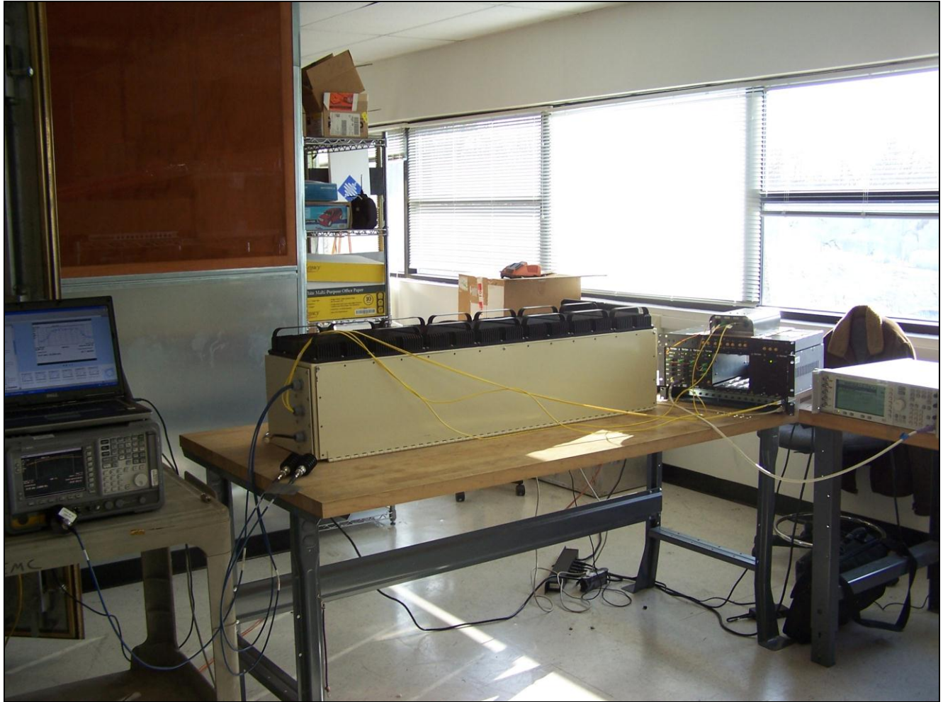
Photograph 4. Occupied Bandwidth, Test Setup
