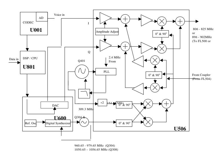
Figure 4-3: Transmitter Modulation System
