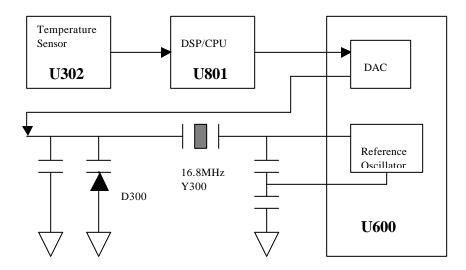
Figure 4-1: 16.8 MHz Reference Oscillator
