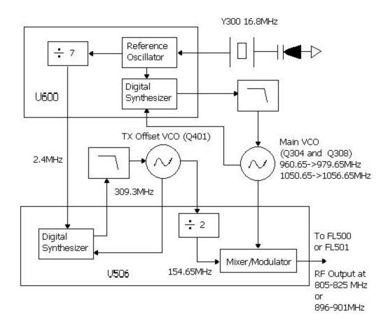
Figure 4-2: Transmitter Frequency Generation
