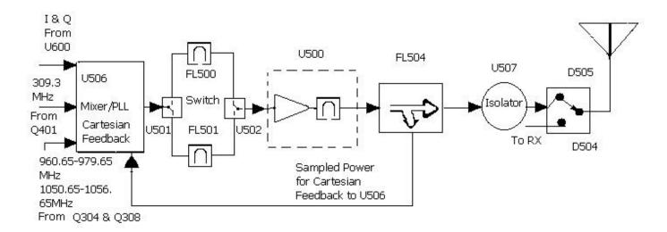
Figure 4-4: Transmitter Front Stage Line-Up
