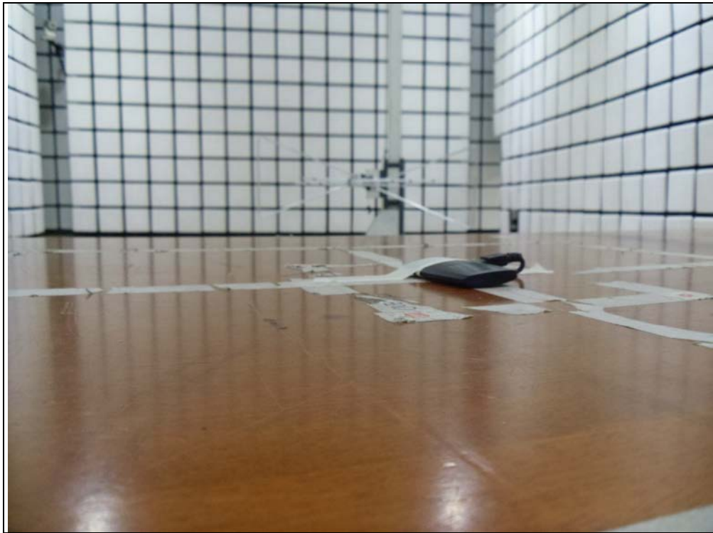
Photo of Field Strength & Spurious Emission Test(Below 1 GHz)
