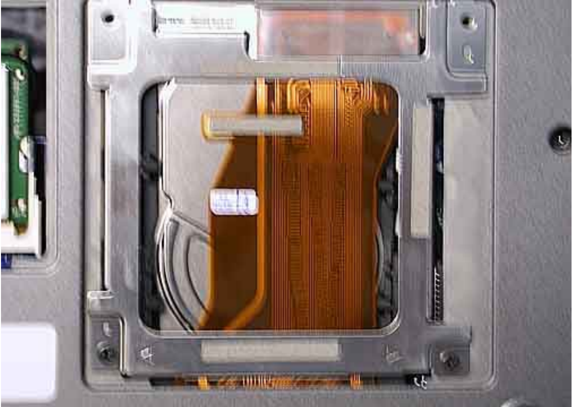
LE1600 HDD Location
