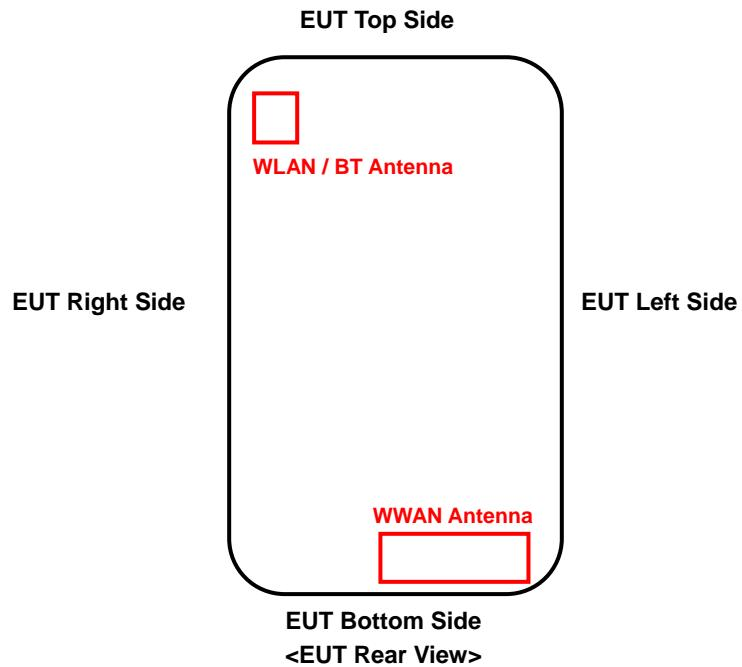
The separation distance for antenna to edge:
