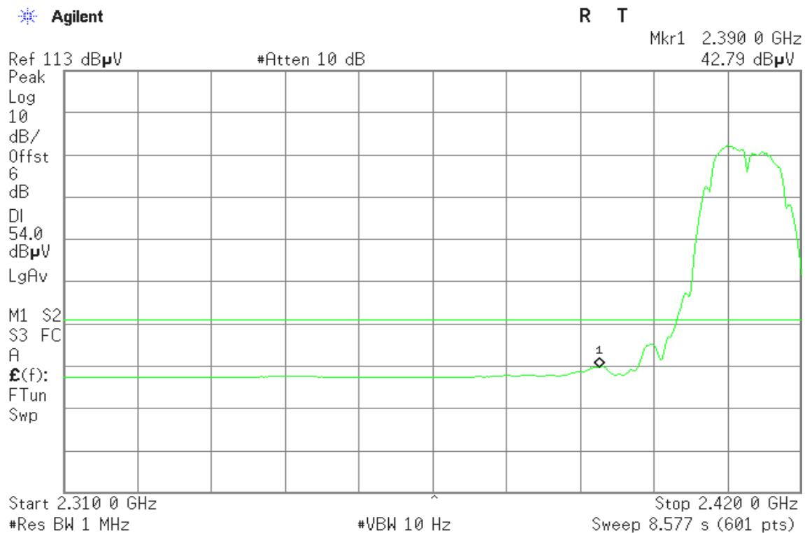
**Band Edges (IEEE 802.11b / CH High)****Detector mode: Peak****Polarity: Vertical**
