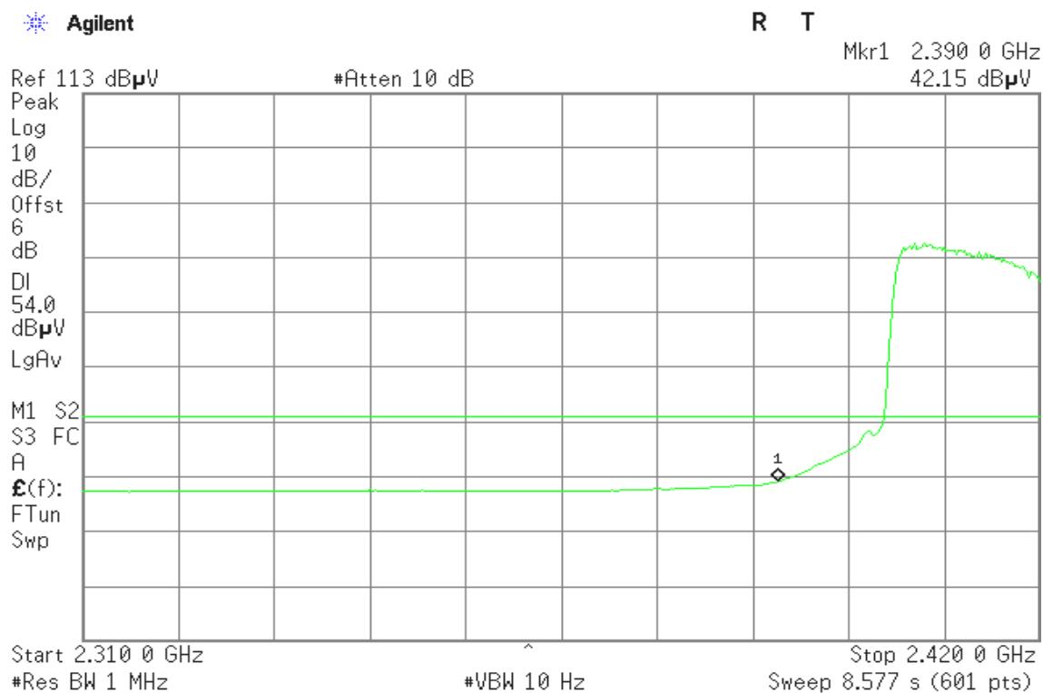
**Band Edges (IEEE 802.11g / CH High)****Detector mode: Peak****Polarity: Vertical**
