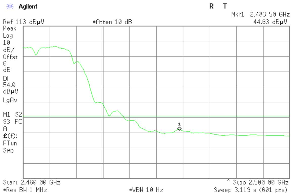
**Band Edges (IEEE 802.11g / CH Low)****Detector mode: Peak****Polarity: Vertical**
