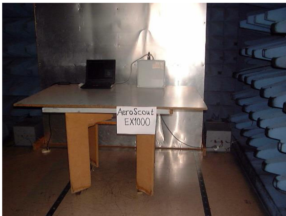
Figure 1. Conducted Emission Test.
