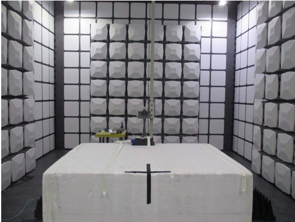
Description: Front View of Radiated Emission Test Setup (Above 1GHz)
