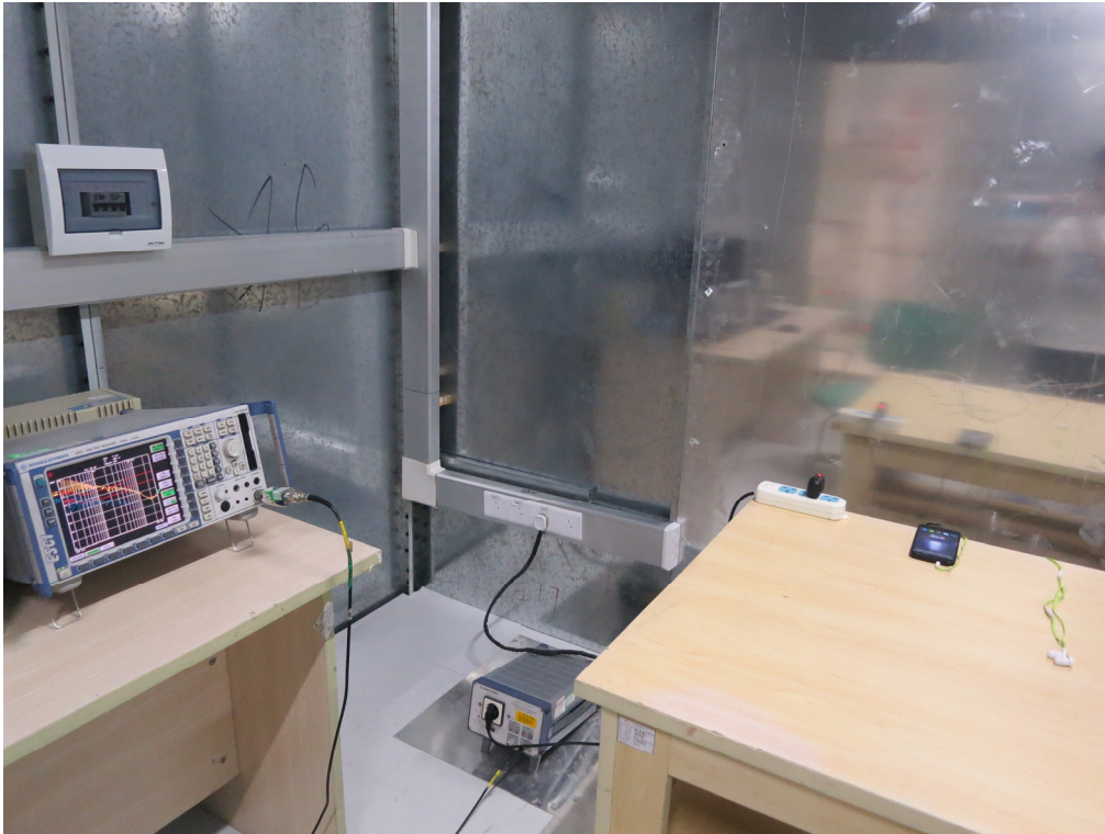
FCC RADIATED EMISSION TEST SETUP
