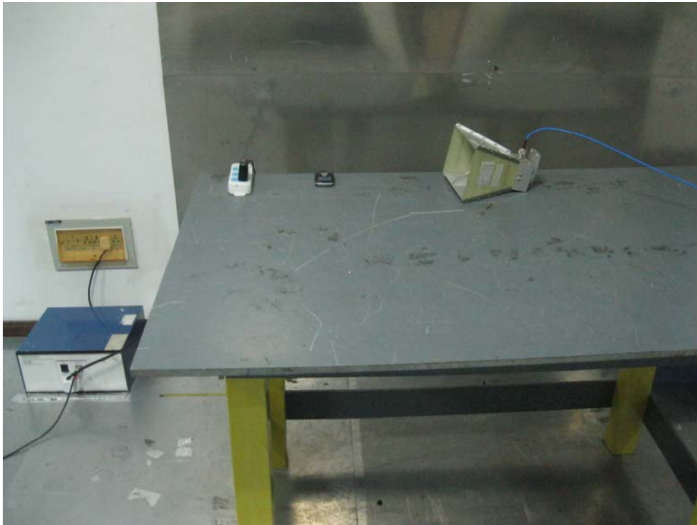
Conducted Emissions Test Setup - Front View
