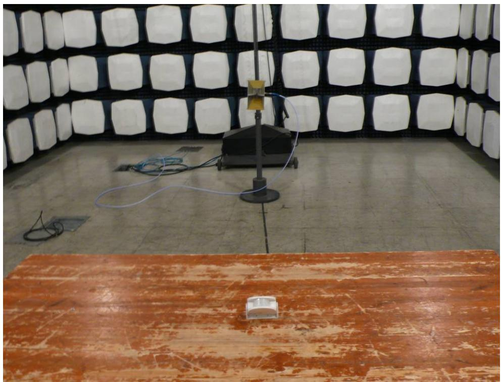
Measurement of Radiated Emission Test 1GHz-5GHz
