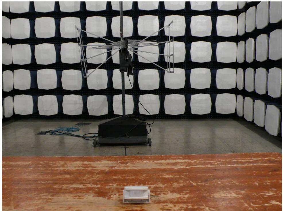
Measurement of Radiated Emission Test
