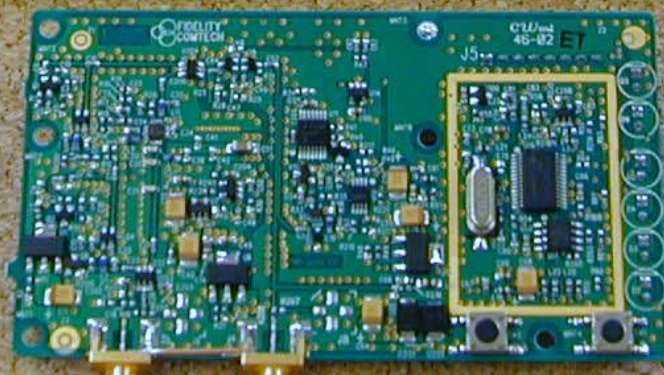
FCI-2451 Amplified Antenna (Witch's Hat) - Case Open - Amplifier Removed
