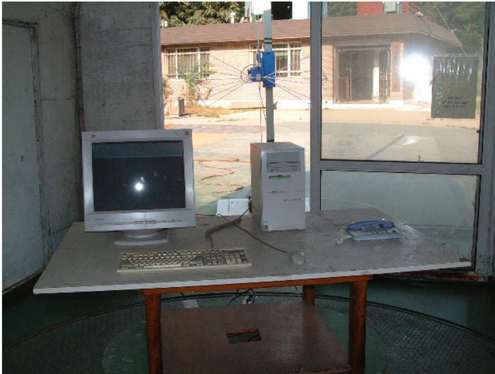
RADIATED EMISSION SETUP PHOTOGRAPH - FRONT VIEW ( 30 - 300 MHz )
