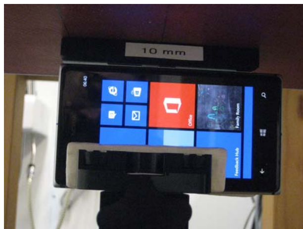
Photo of the device positioned for WR mode measurement – right edge facing phantom. The spacer was removed before the start of the measurements.
