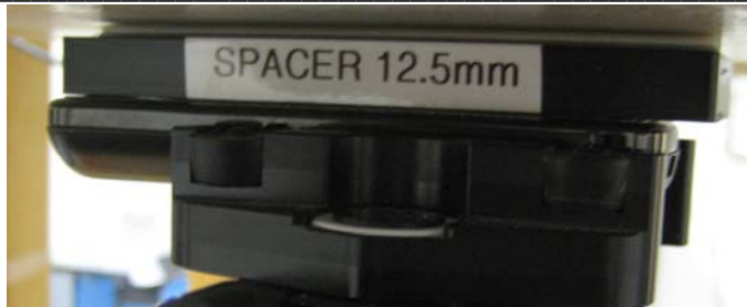
Photo of the device positioned for WR mode measurement – display facing phantom. The spacer was removed before the start of the measurements.
