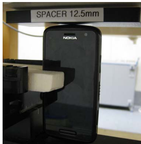
Photo of the device positioned for WR mode measurement – top edge facing phantom. The spacer was removed before the start of the measurements.
