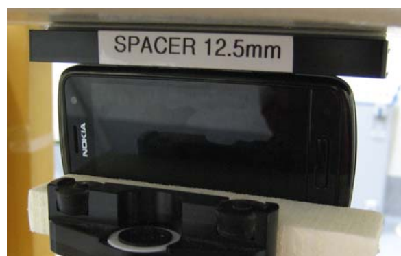
Photo of the device positioned for WR mode measurement – right edge facing phantom. The spacer was removed before the start of the measurements.
