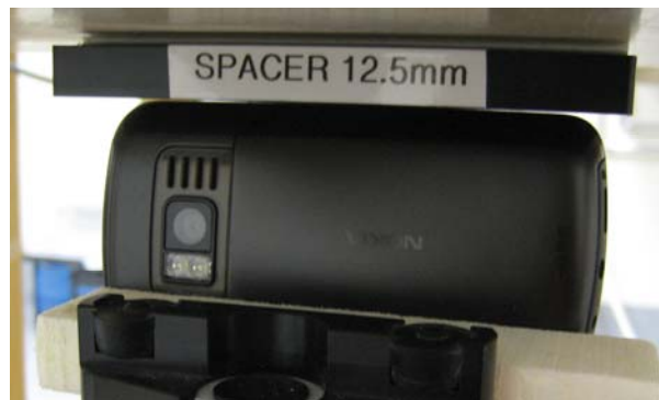
Photo of the device positioned for WR mode measurement – left edge facing phantom. The spacer was removed before the start of the measurements.
