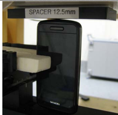
Photo of the device positioned for WR mode measurement – bottom edge facing phantom. The spacer was removed before the start of the measurements.
