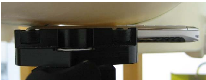
Photo of the device in “cheek” position
