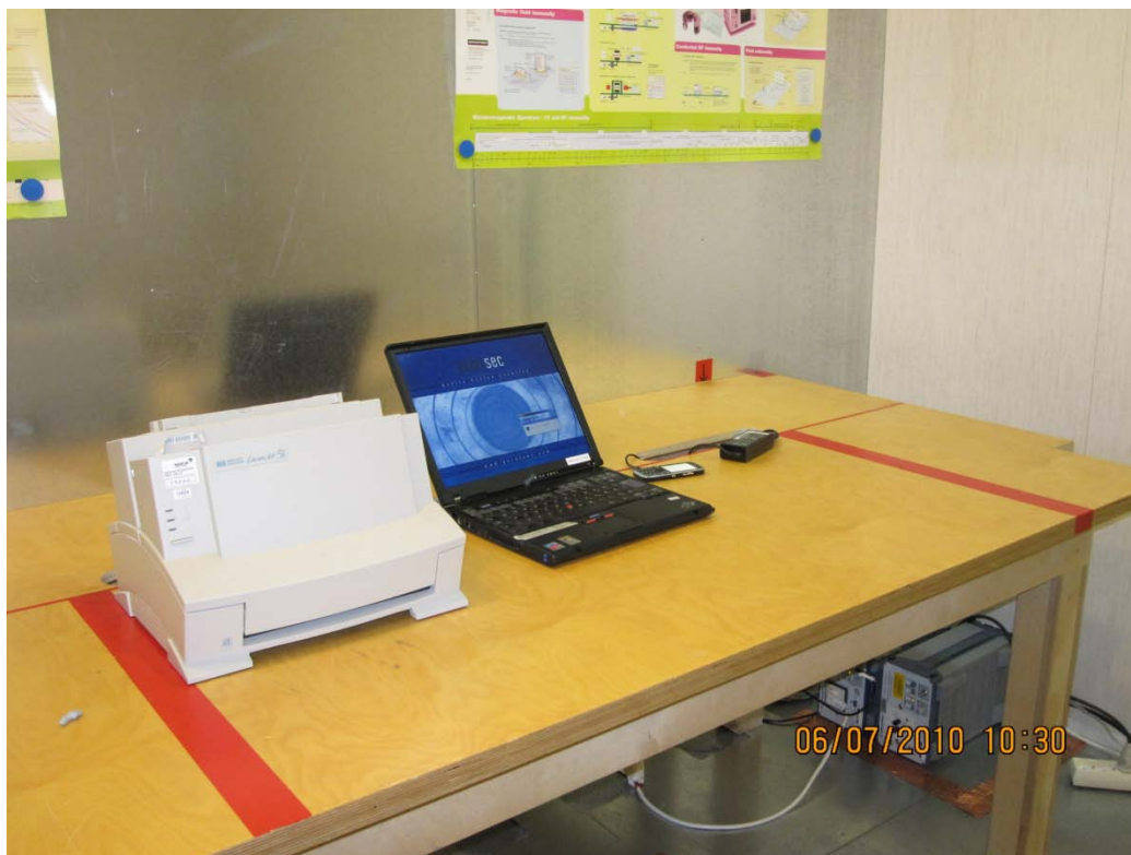
Picture 1 AC powerline conducted emission measurement 15B
