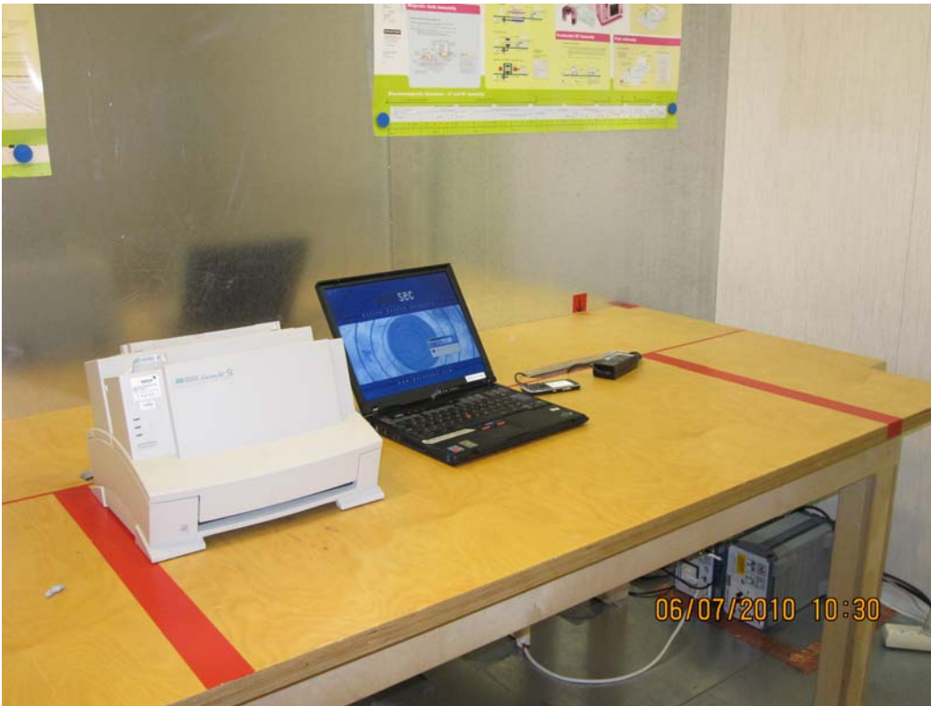
Picture 1 AC powerline conducted emission measurement 15B
