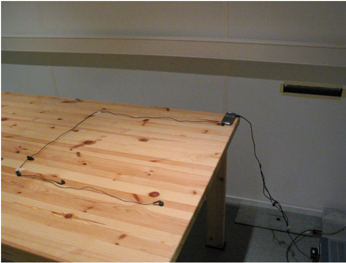
Picture 3 AC powerline conducted emission measurement 15C
