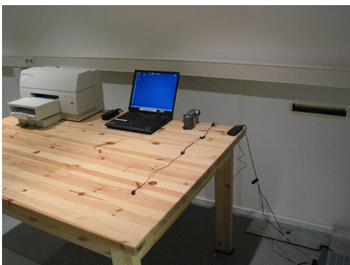
Picture 4 AC powerline conducted emission measurement GSM RX / Bluetooth TX / WLAN RX+ Computer peripherals
