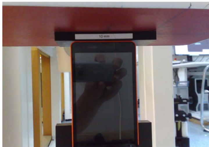
Photo of the device positioned for WR mode measurement – bottom edge facing phantom. The spacer was removed before the start of the measurements.
