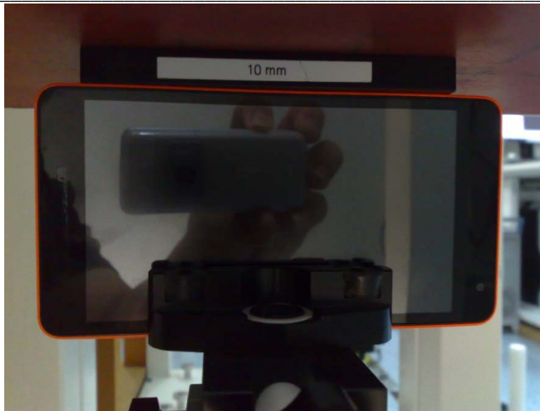
Photo of the device positioned for WR mode measurement – left edge facing phantom. The spacer was removed before the start of the measurements.
