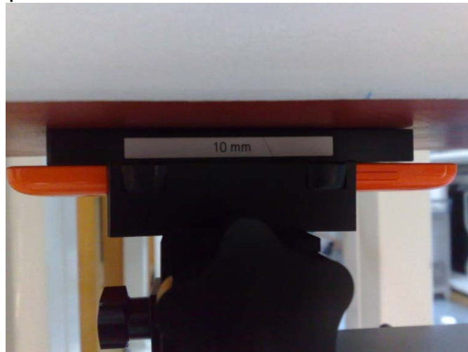
Photo of the device positioned for WR mode measurement – display facing phantom. The spacer was removed before the start of the measurements.
