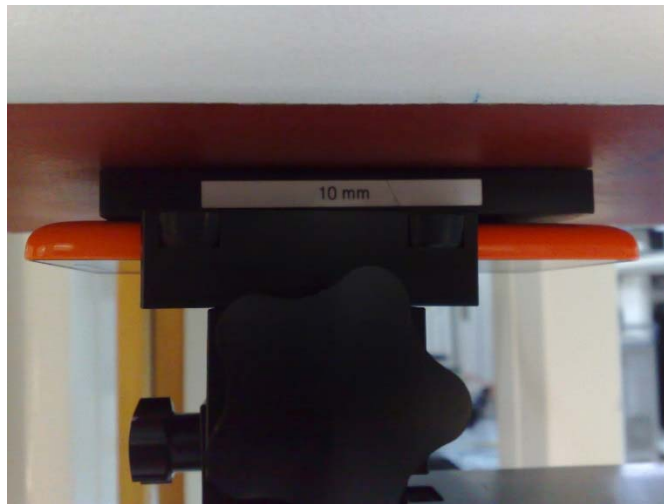
Photo of the device positioned for WR mode measurement –back facing phantom. The spacer was removed before the start of the measurements.
