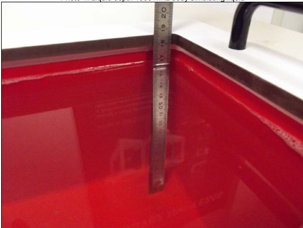
Photo 4: Liquid depth 1900 MHz body simulating liquid
