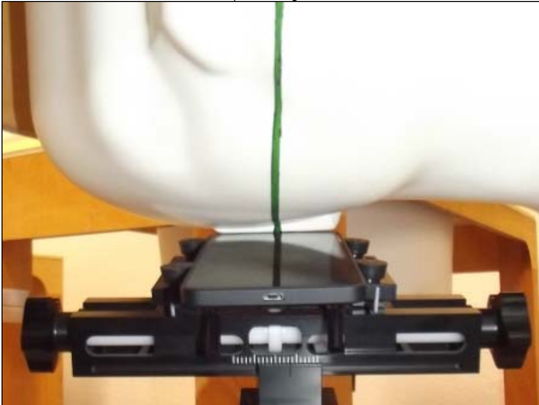
Photo 16: Test position right hand tilted 15°
