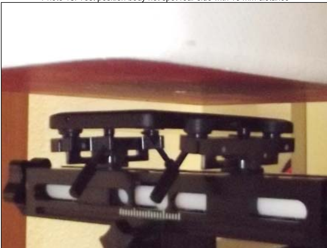
Photo 18: Test position body hot spot rear side with 10 mm distance
