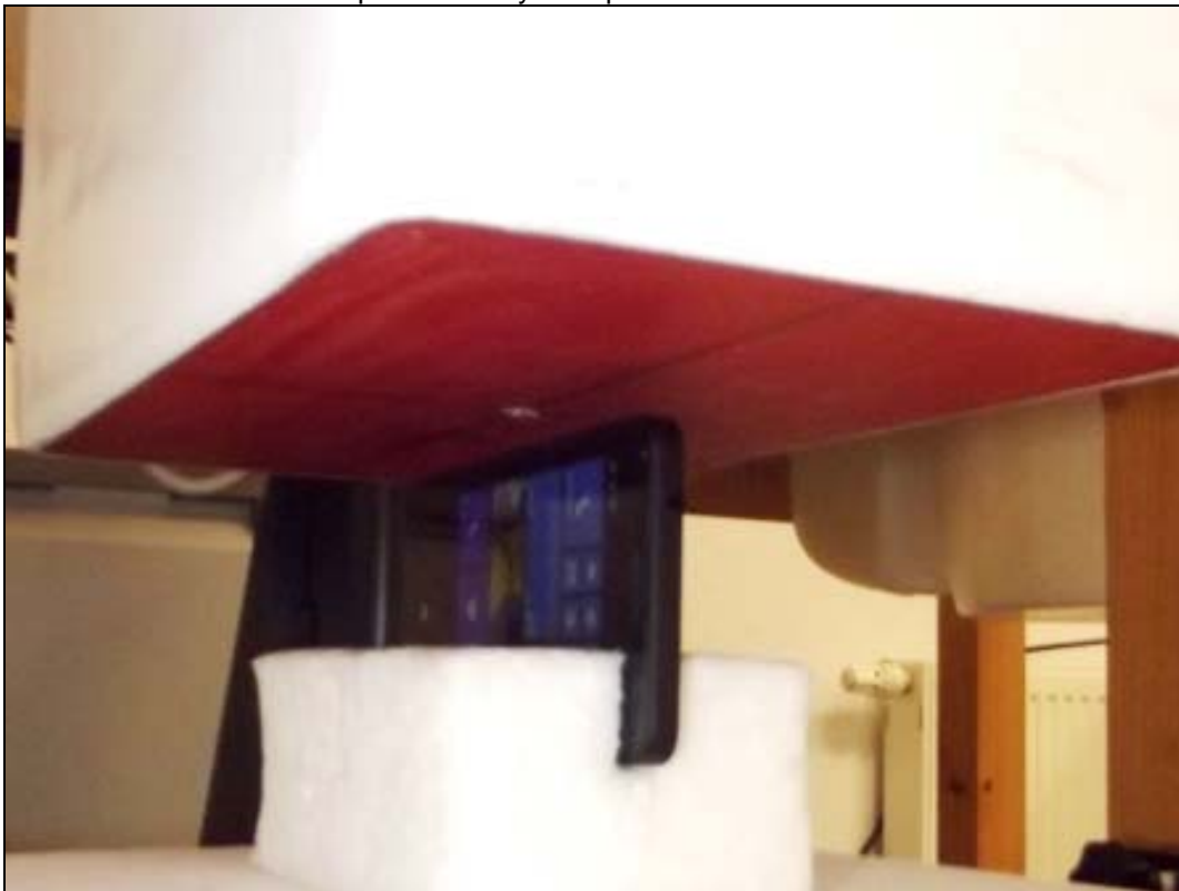
Photo 19: Test position body hot spot left side with 10 mm distance
