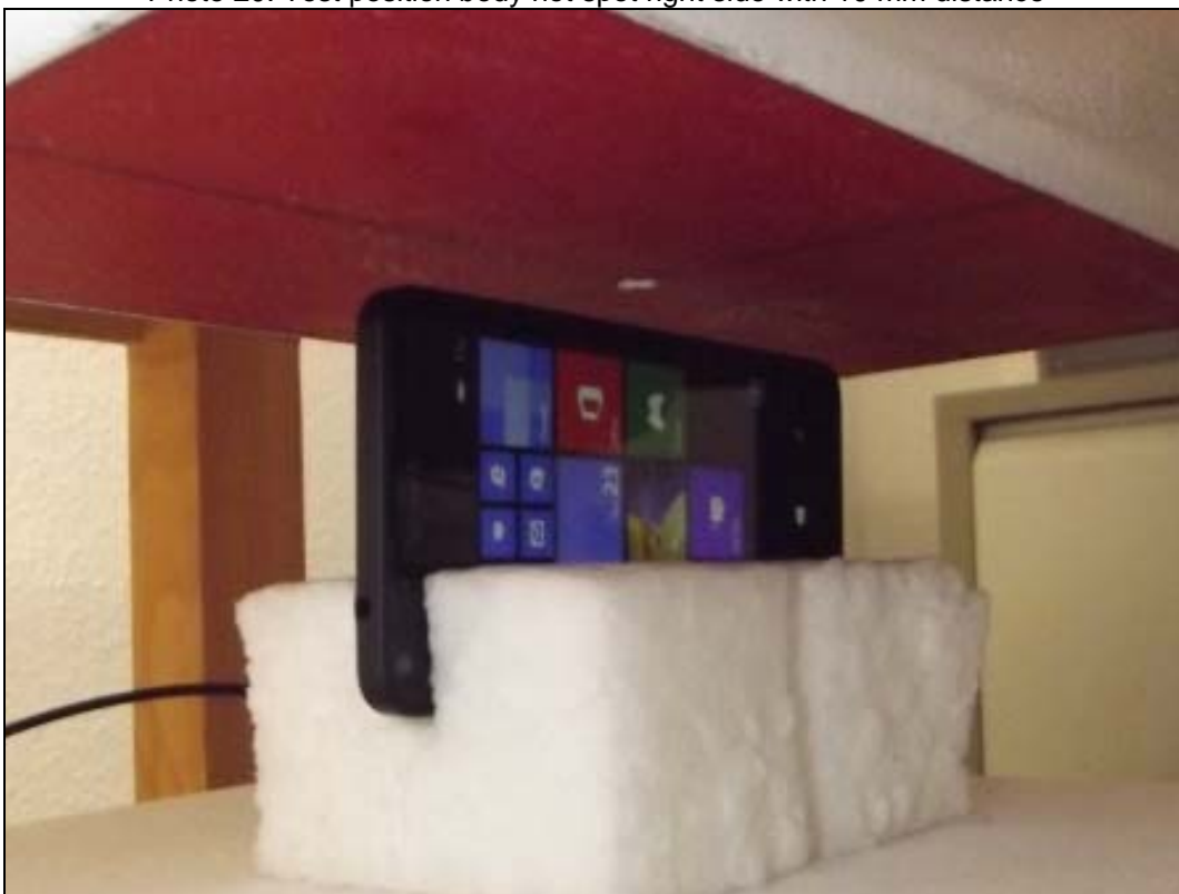
Photo 20: Test position body hot spot right side with 10 mm distance
