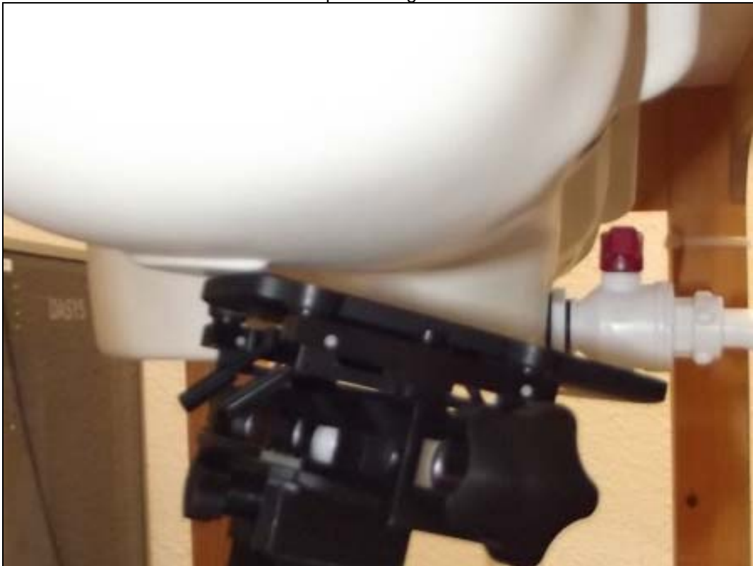
Photo 16: Test position right hand tilted 15°
