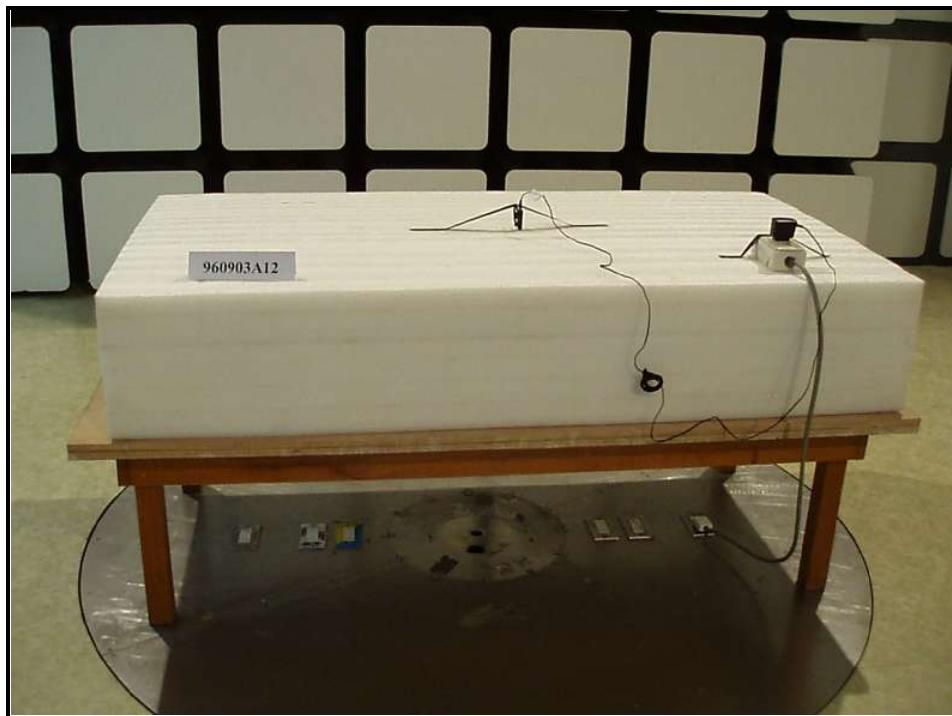
RADIATED EMISSION TEST (Mode B)
