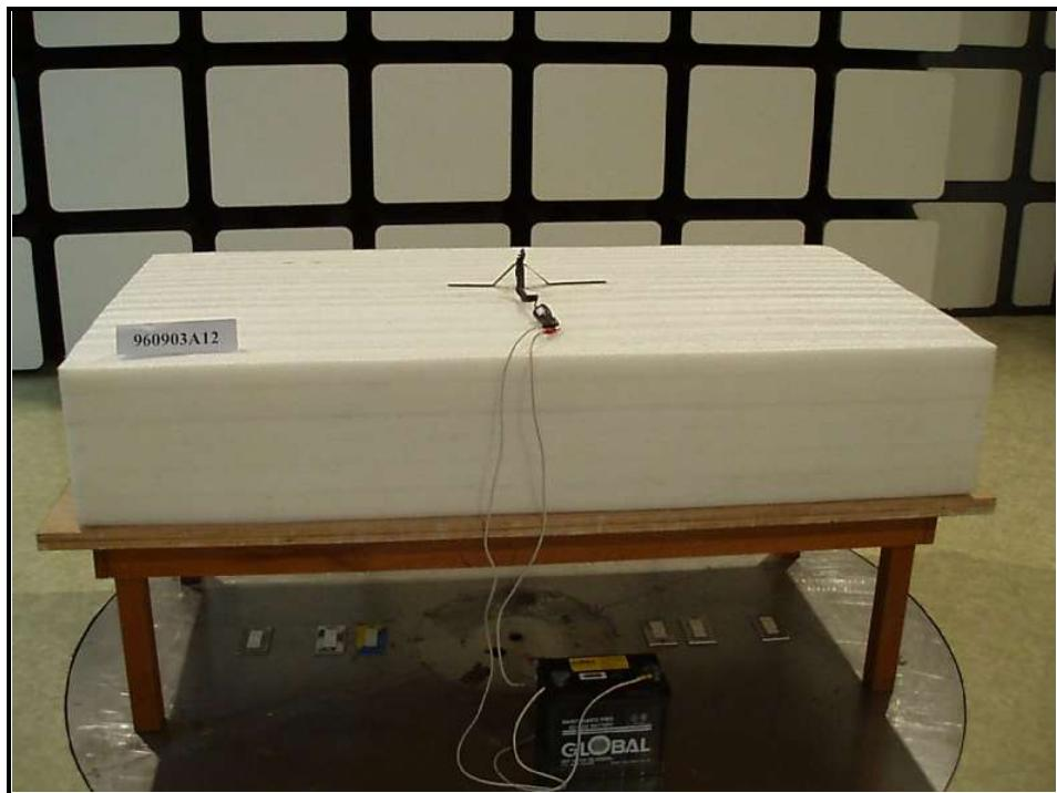
RADIATED EMISSION TEST (Mode C)
