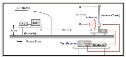
Above 1GHz Test Setup:
