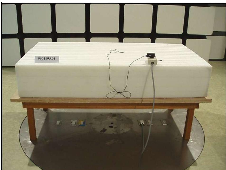
RADIATED EMISSION TEST (For Mode B)
