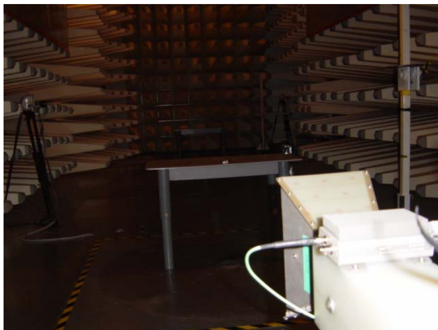
Set-up for Radiation Emission (reference photo)
