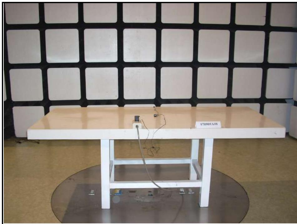
RADIATED EMISSION TEST (Mode B)
