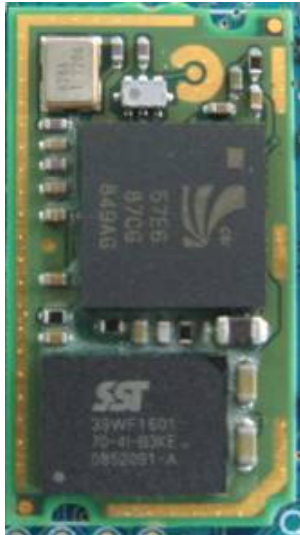
<Bluetooth Module of Top PCB>
