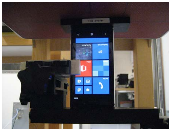
Photo of the device positioned for WR mode measurement – bottom edge facing phantom. The spacer was removed before the start of the measurements.
