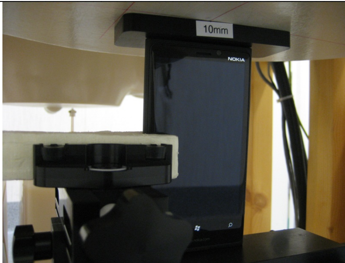
Photo of the device positioned for WR mode measurement – top edge facing phantom. The spacer was removed before the start of the measurements.
