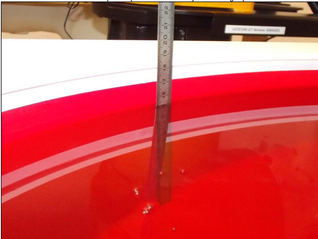
Photo 2: Liquid depth 850 MHz body simulating liquid
