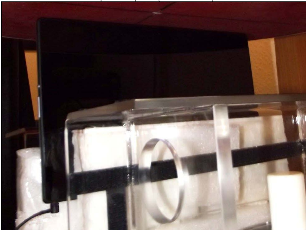
Photo 10: Test position top side (15mm distance) with headset
