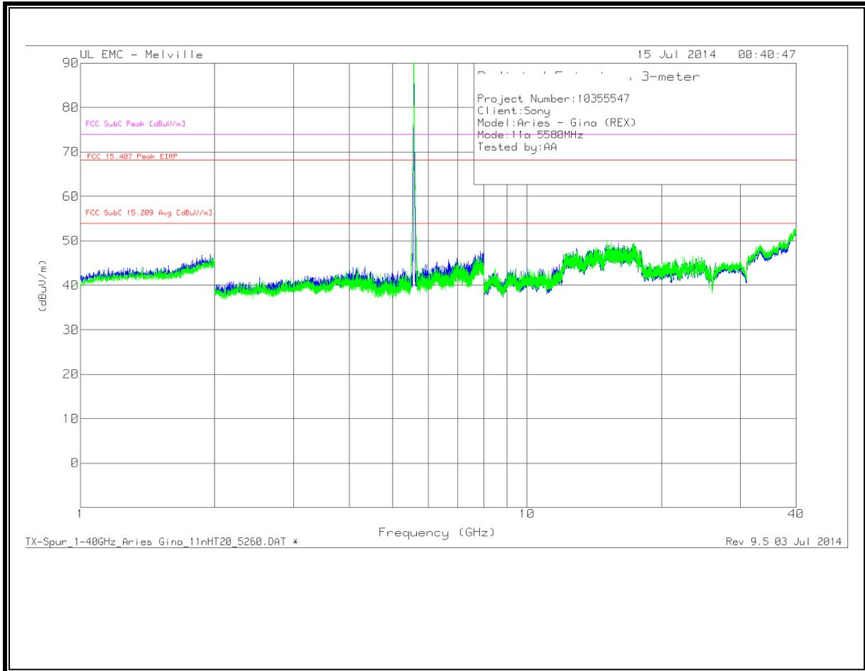
Note: Emission was scanned up to 40GHz; No emissions were detected above the noise floor.
