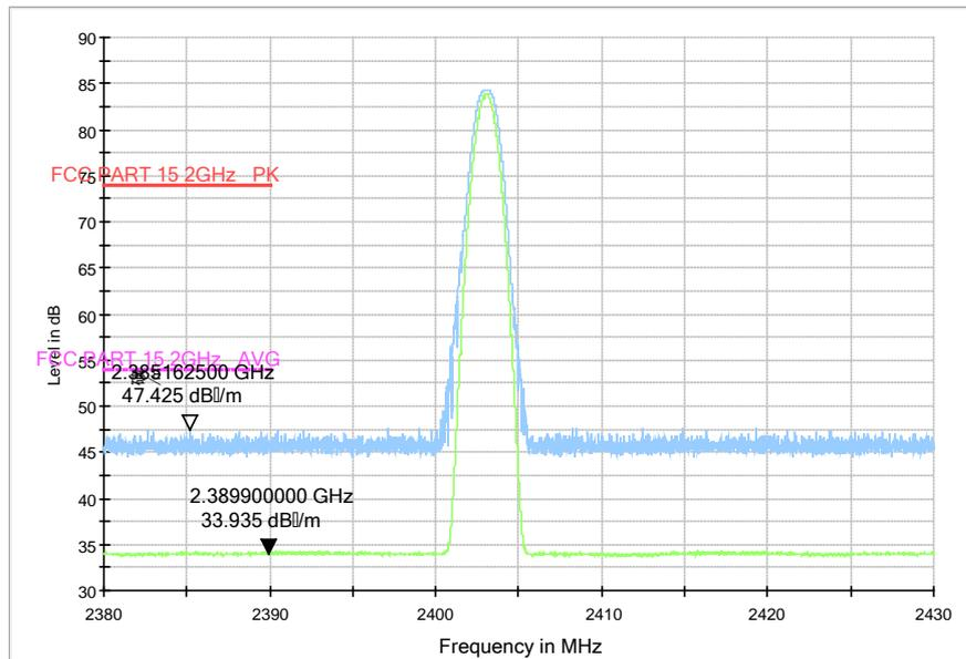
Fig.12. Radiated emission (Power): Low Channel
