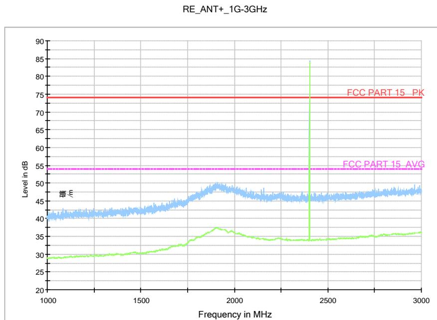
Fig.4. Radiated emission: Channel 0, 1 GHz - 3 GHz
