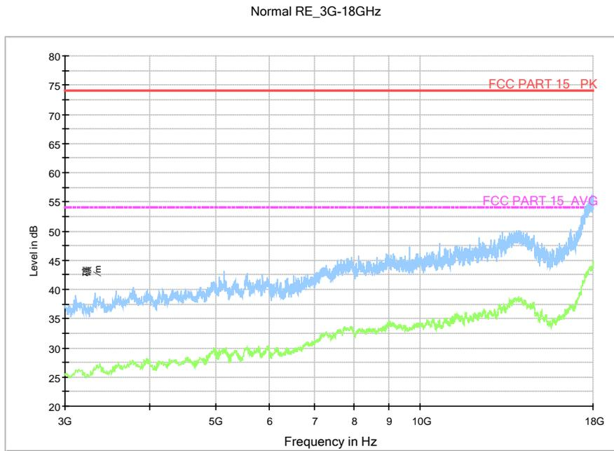
Fig.5. Radiated emission: Channel 0, 3 GHz - 18 GHz
