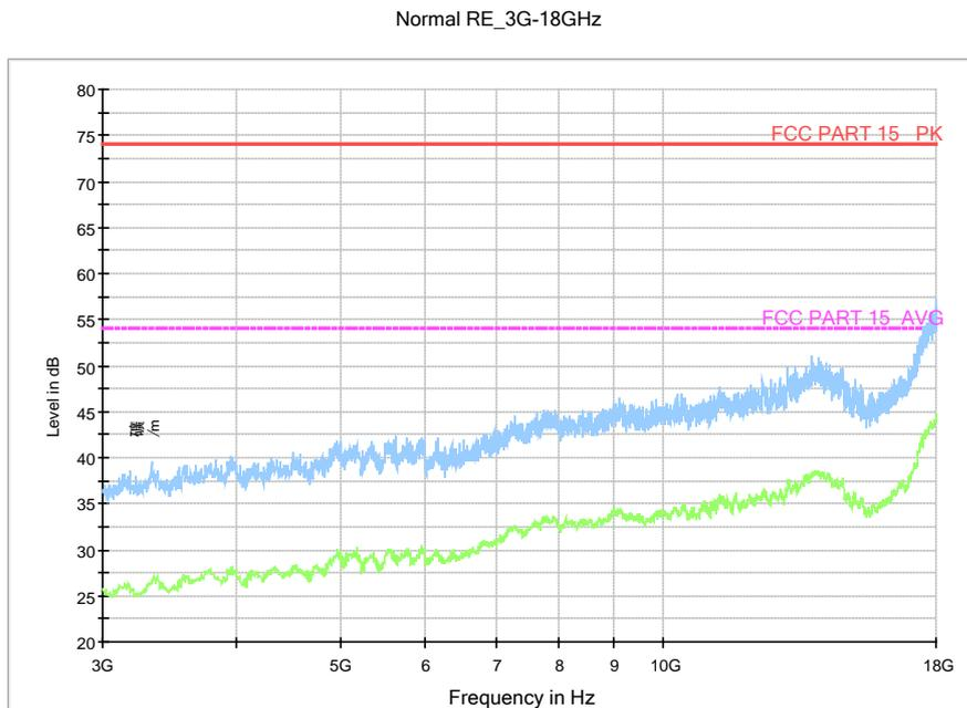
Fig.8. Radiated emission: Channel 39, 3 GHz - 18 GHz
