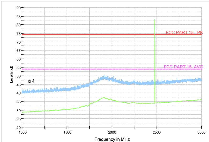
Fig.10. Radiated emission: Channel 78, 1 GHz - 3 GHz
