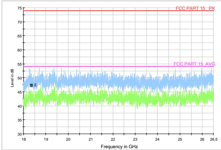
Fig.9. Radiated emission: Channel 39, 18 GHz ~ 26 GHz
