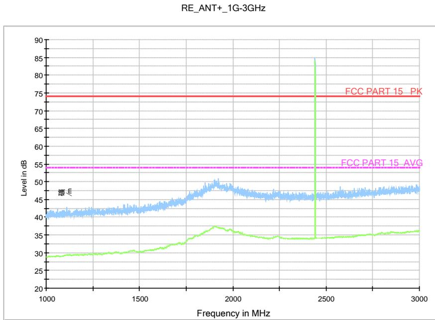
Fig.7. Radiated emission: Channel 39, 1 GHz - 3 GHz
