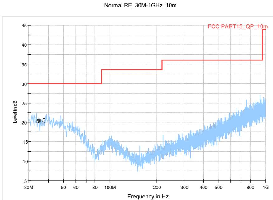
Fig.6. Radiated emission: Channel 39, 30 MHz - 1 GHz
