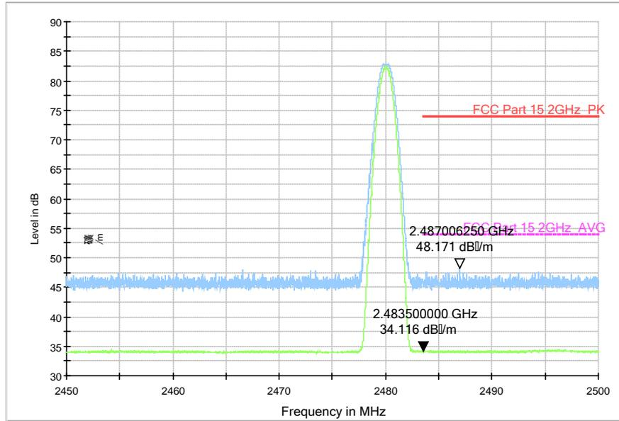
Fig.13. Radiated emission (Power): High Channel
